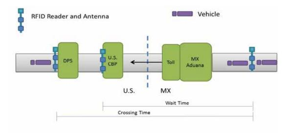
FIGURE 14 Border crossing radio frequency identification system. (Source: Texas A&M Transportation Institute.)
