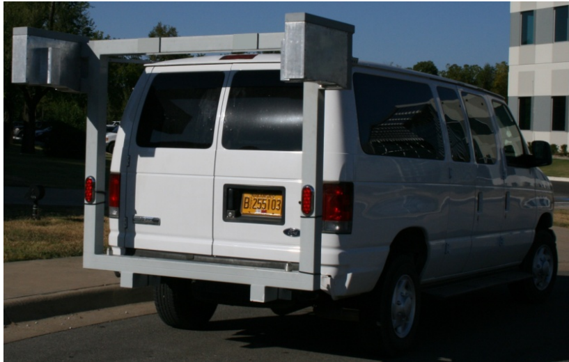
Figure 7. The Prototype DHDV with Two 2D/3D Hybrid Sensor Cases of PaveVision3D
