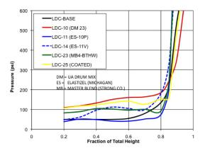
Figure 9.3 Drum Mix Stress-Strain Material Behavior
