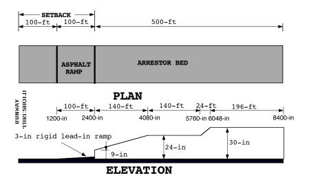
Figure 7.1. Arrestor Bed Configuration
