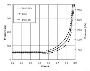
Figure 7.2. Low-Density Concrete Material Behavior
