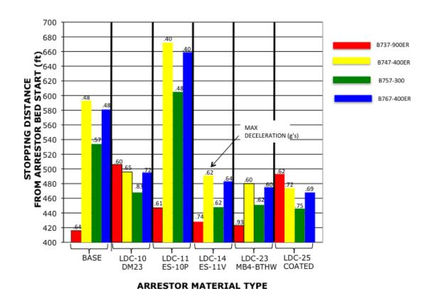
Figure 9.4 Stopping Distance as a Function of Drum Mix (Runway Safety Area Entry Vel. = 70 knots, 0 Reverse Thrust)
