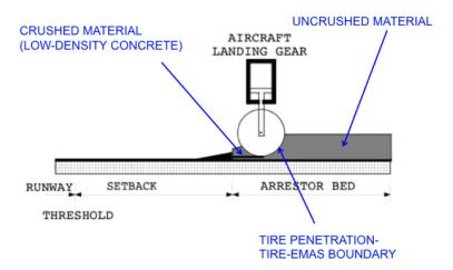
Figure 1.1. Aircraft Movement Through an EMAS
