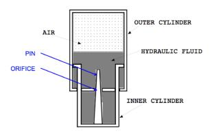
Figure 5.1. Oleo-Pneumatic Strut
