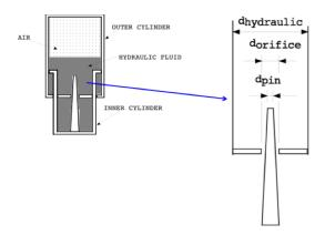
Figure 5.3. Hydraulic Strut Force
