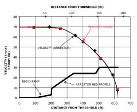
Figure 8.1. SGAS Calibration with ARRESTOR Using Stopping Distance
