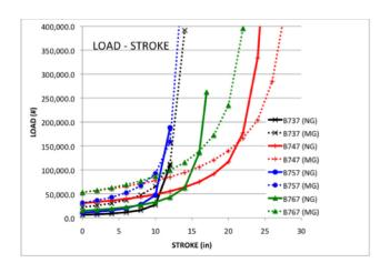
Figure 6.5. Load-Stroke Behavior used as SGAS Input
