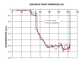
Figure 8.2. SGAS Comparison with ARRESTOR for Aircraft Deceleration
