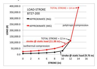
Figure 6.3. B727 Approximate Load-Stroke Behavior
