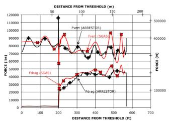
Figure 8.4. SGAS Comparison with ARRESTOR for Main Gear Strut Forces
