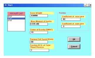
Figure 4.7. ARRESTOR Select Aircraft Pop-Up Window.
