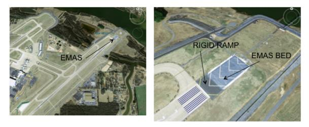
Figure 1.2. Installed EMAS at Adams Field; Little Rock, AR
