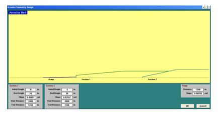
Figure 4.6 EMAS Geometry Pop-Up Window.
