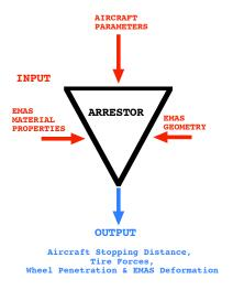
Figure 4.3. FAA ARRESTOR Input – Output
