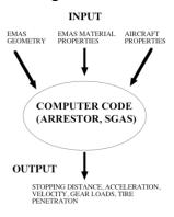
Figure 4.1. Numerical Analysis Input-Output Format.
