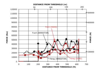
Figure 8.3. SGAS Comparison with ARRESTOR for Nose Gear Strut Forces
