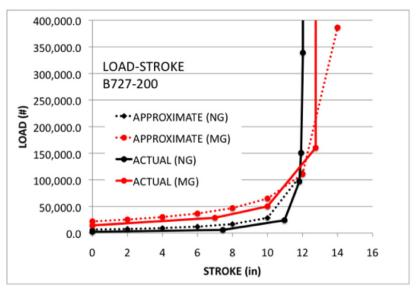
Figure 6.4. B727 Load-Stroke Behavior Comparing Approximate and Actual
