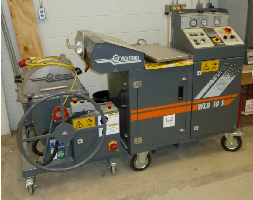
Figure 7 – Wirtgen WLM 30 mixer (left) and Wirtgen WLB 10 S foaming machine (right)
