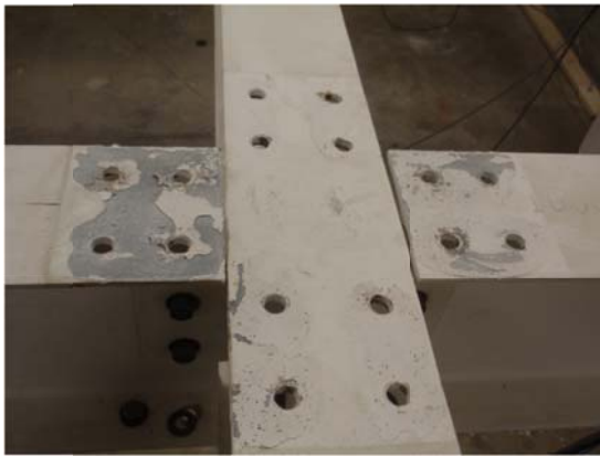
Figure 6.22: Damage Case #3 – Removal of Gusset Plates
