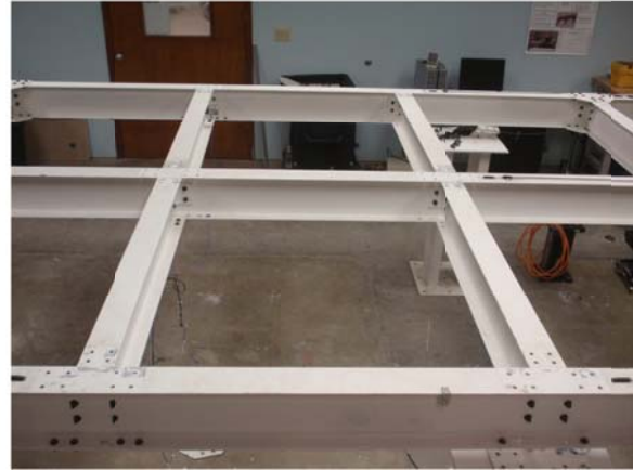
Figure 6.22: Damage Case #3 – Removal of Gusset Plates
