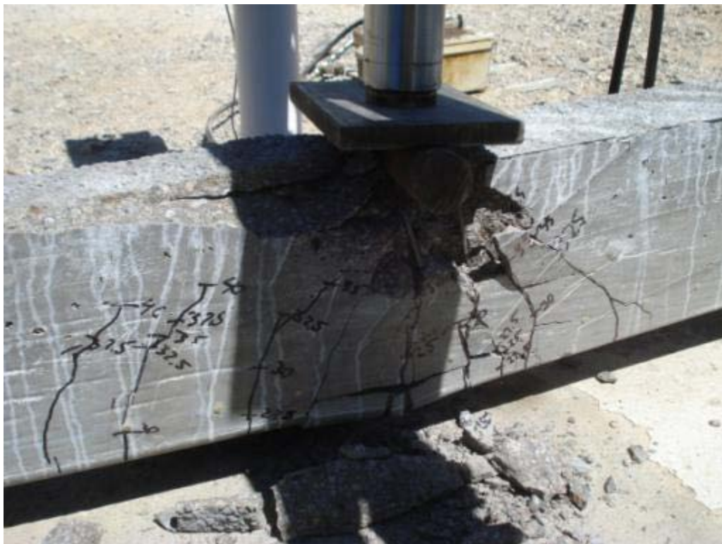
Figure 6.58: Cracking and failure of specimen HSC-2D
