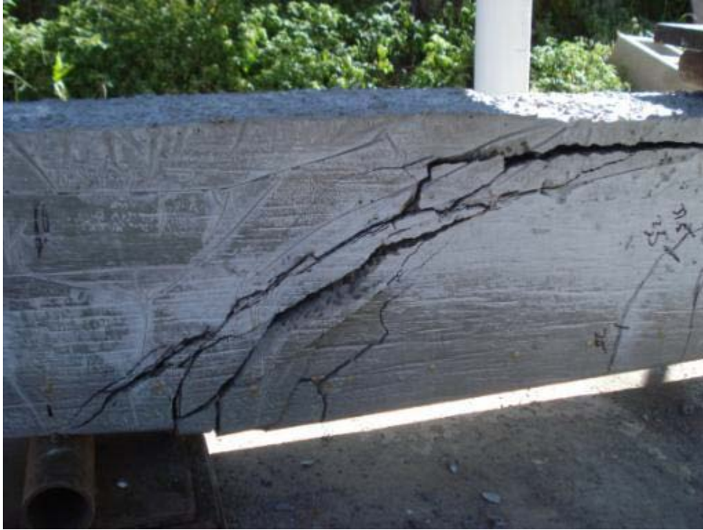
Figure 6.69: Shear cracking of specimen HSS-1D
