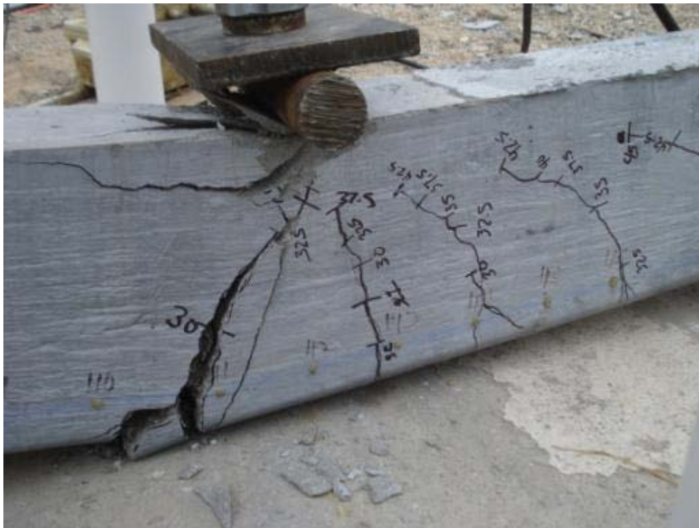
Figure 6.91: Cracking and failure of specimen HSL-2L
