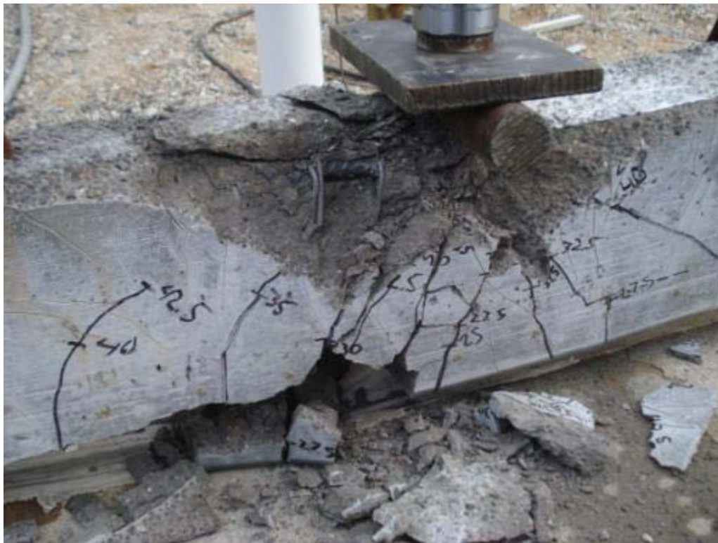
Figure 6.73: Cracking and failure of specimen HSS-2D
