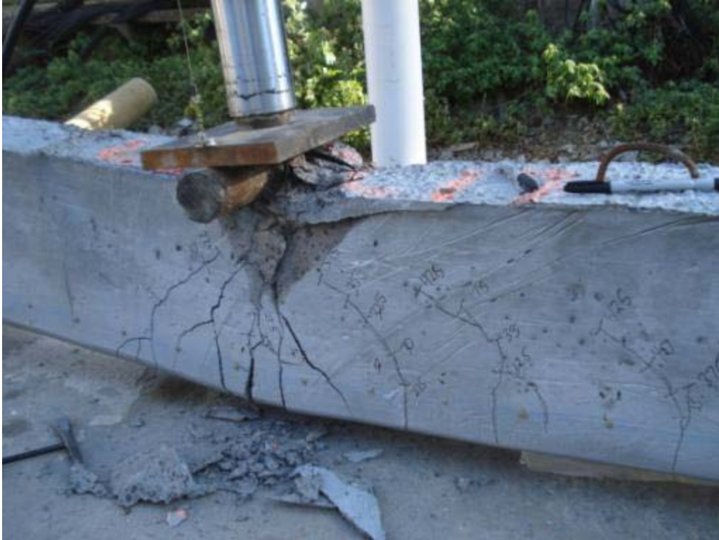
Figure 6.81: Cracking and failure of specimen HSS-4D
