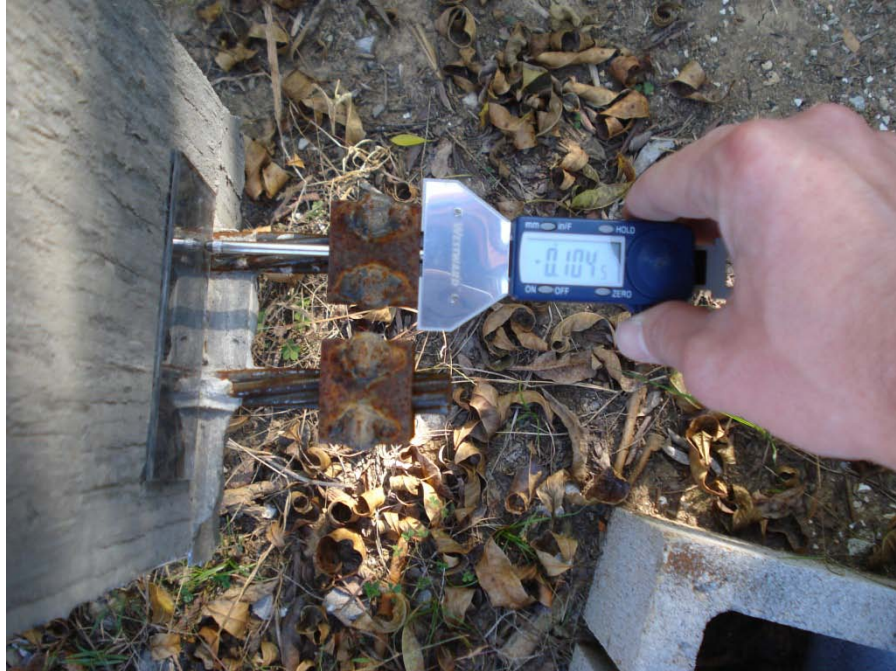
Figure 3.19: Measurement of strand end slip
