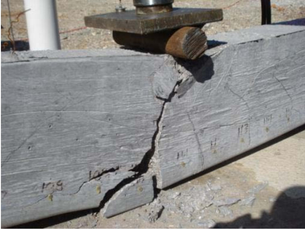
Figure 6.99: Cracking and failure of specimen HSL-4L
