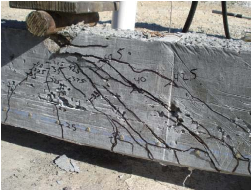
Figure 6.65: Shear failure of specimen HSC-4D
