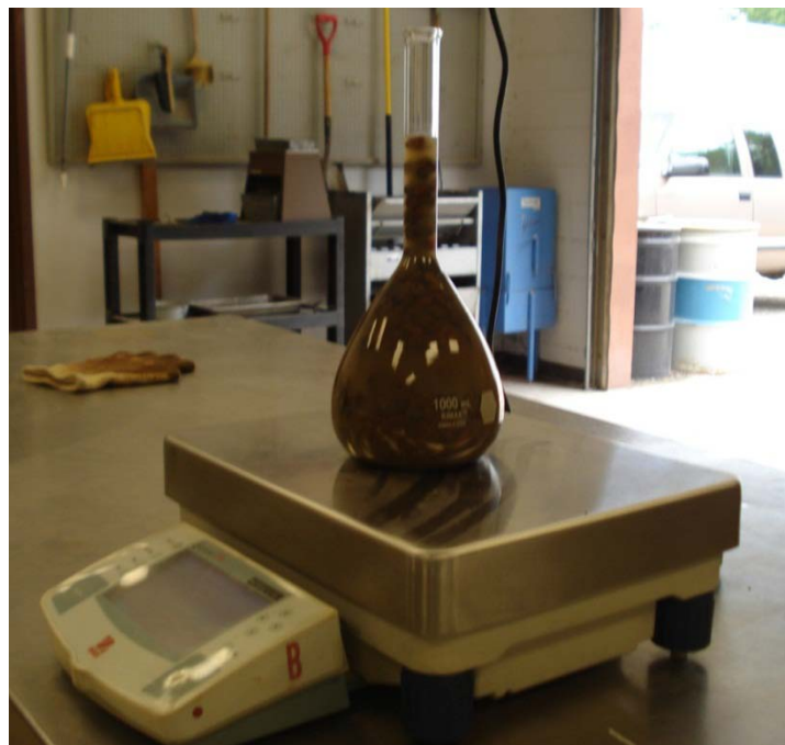
Figure 3.1: Lightweight aggregate specific gravity using the pycnometer method
