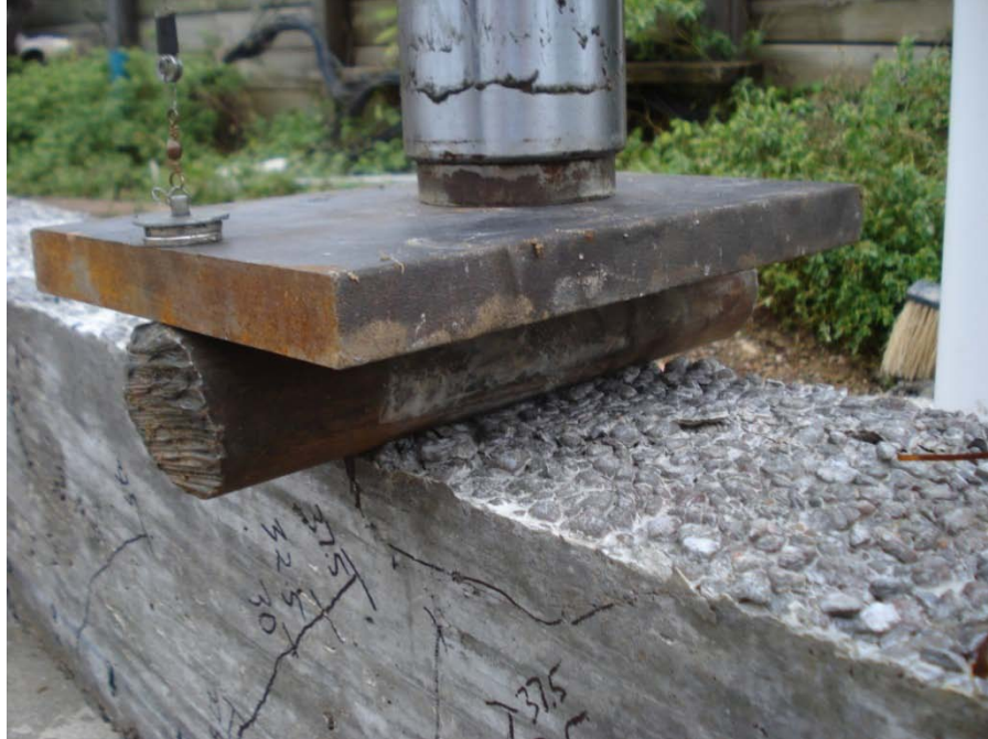
Figure 3.22: Application of point load for flexural testing
