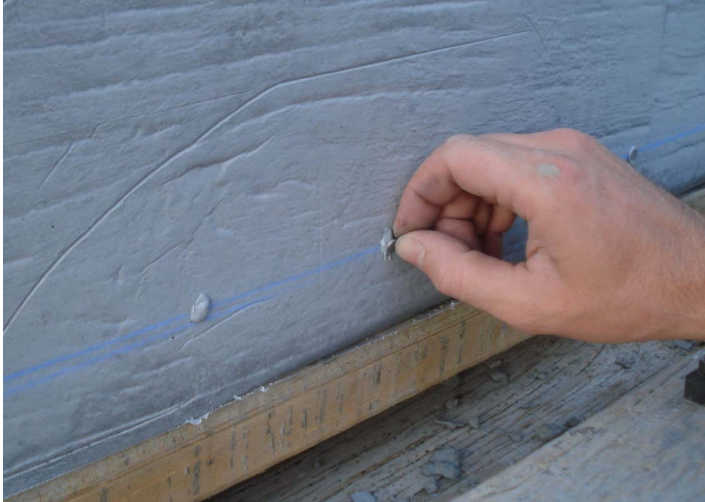
Figure 3.16: Placement of DEMEC points using epoxy
