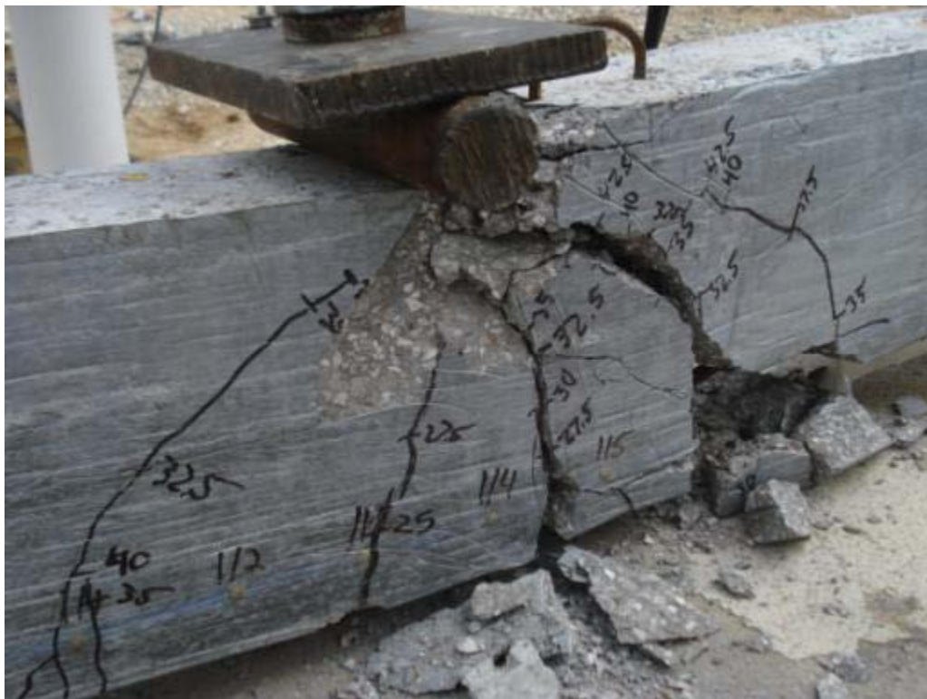
Figure 6.88: Cracking and failure of specimen HSL-1L
