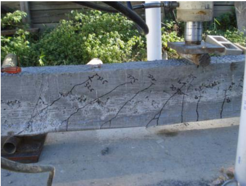
Figure 6.61: Cracking and failure of specimen HSC-3D
