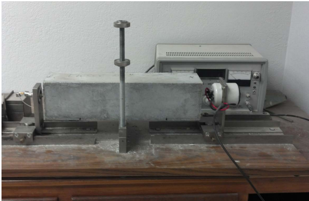
Figure 3.25: Longitudinal fundamental frequency measurement setup
