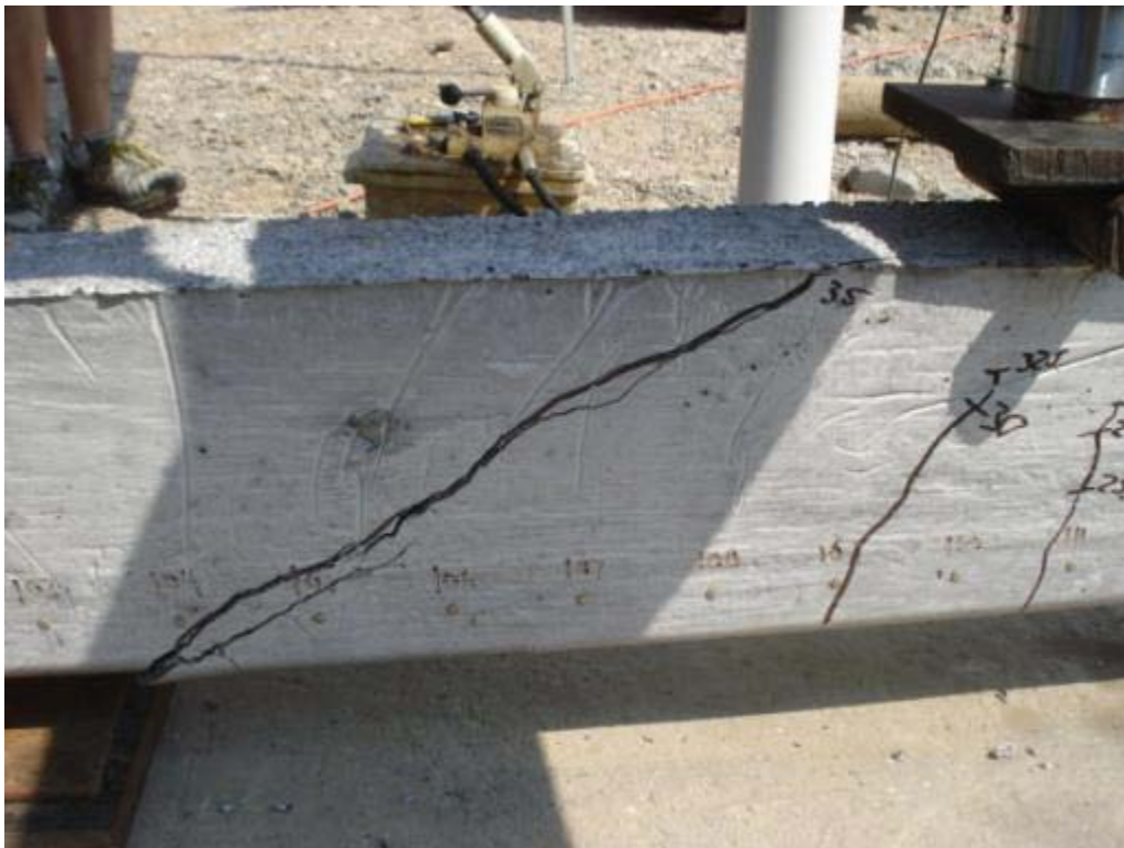
Figure 6.35: Shear cracking of specimen NSS-5L
