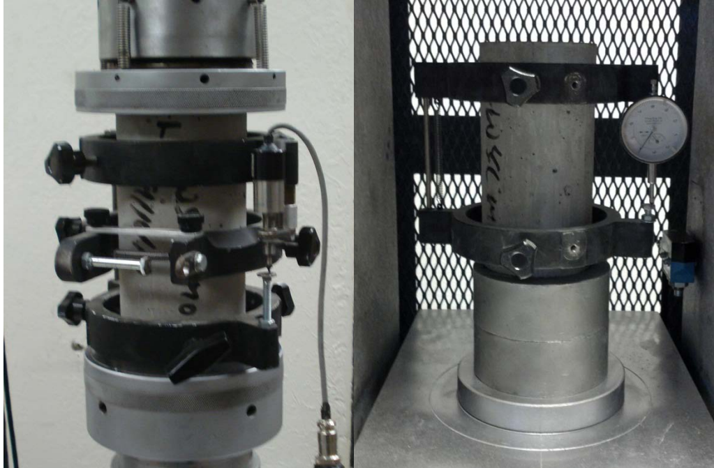
Figure 3.24: Static modulus of elasticity setup using MTS (left) and Forney (right)
