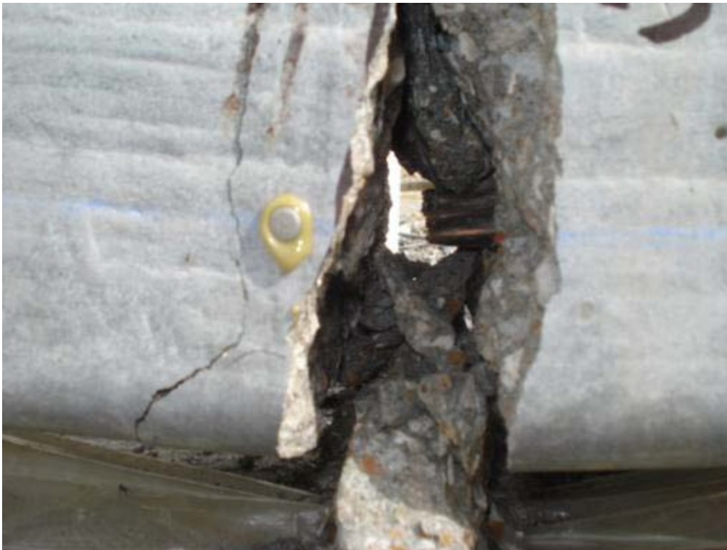
Figure 6.96: Strand fracture at failure of specimen HSL-3L
