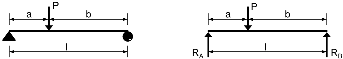
Figure B.1: Beam support conditions and free body diagram for initial shear calculations
