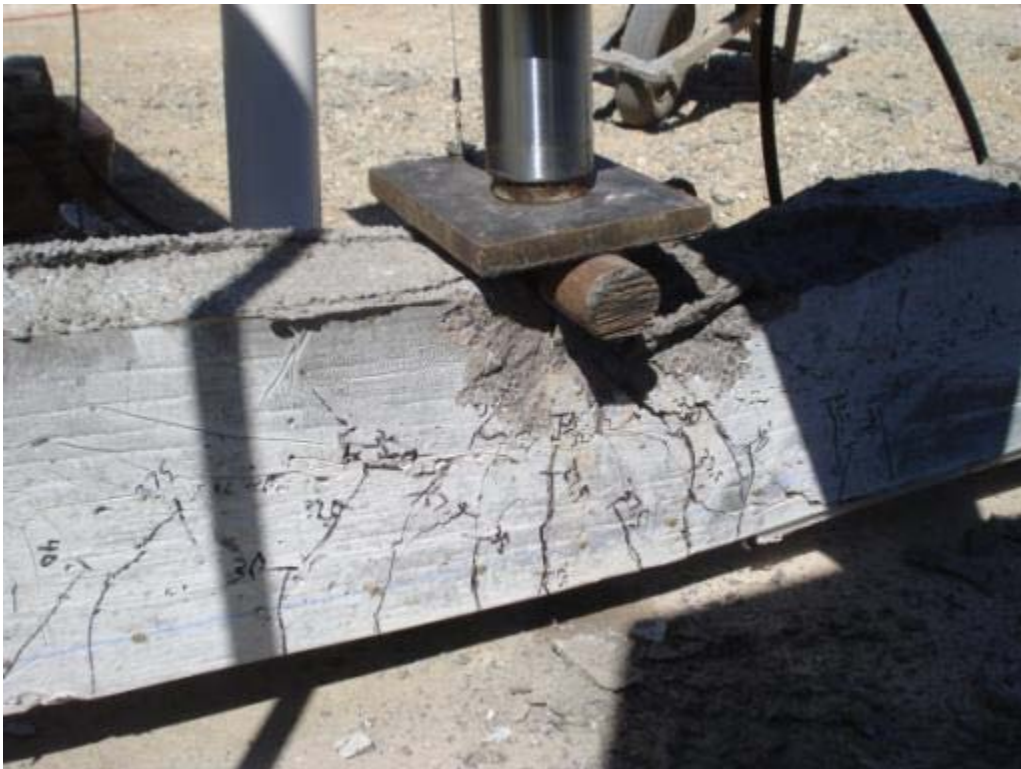
Figure 6.72: Cracking and failure of specimen HSS-1L
