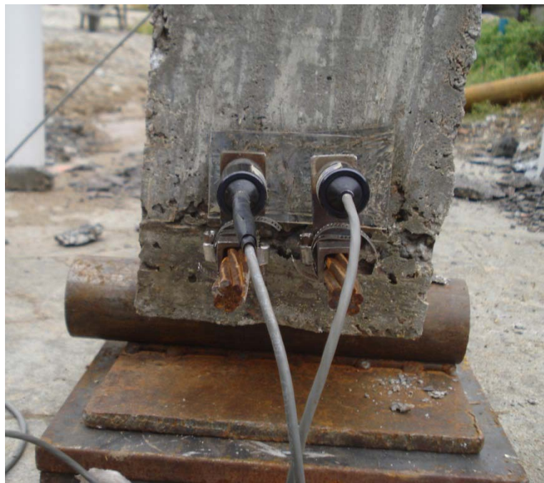
Figure 3.23: Placement of LVDTs to measure strand slip during flexural testing
