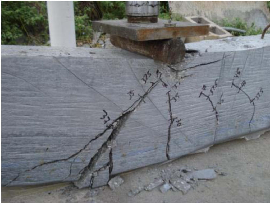
Figure 6.86: Cracking and failure of specimen HSL-1D
