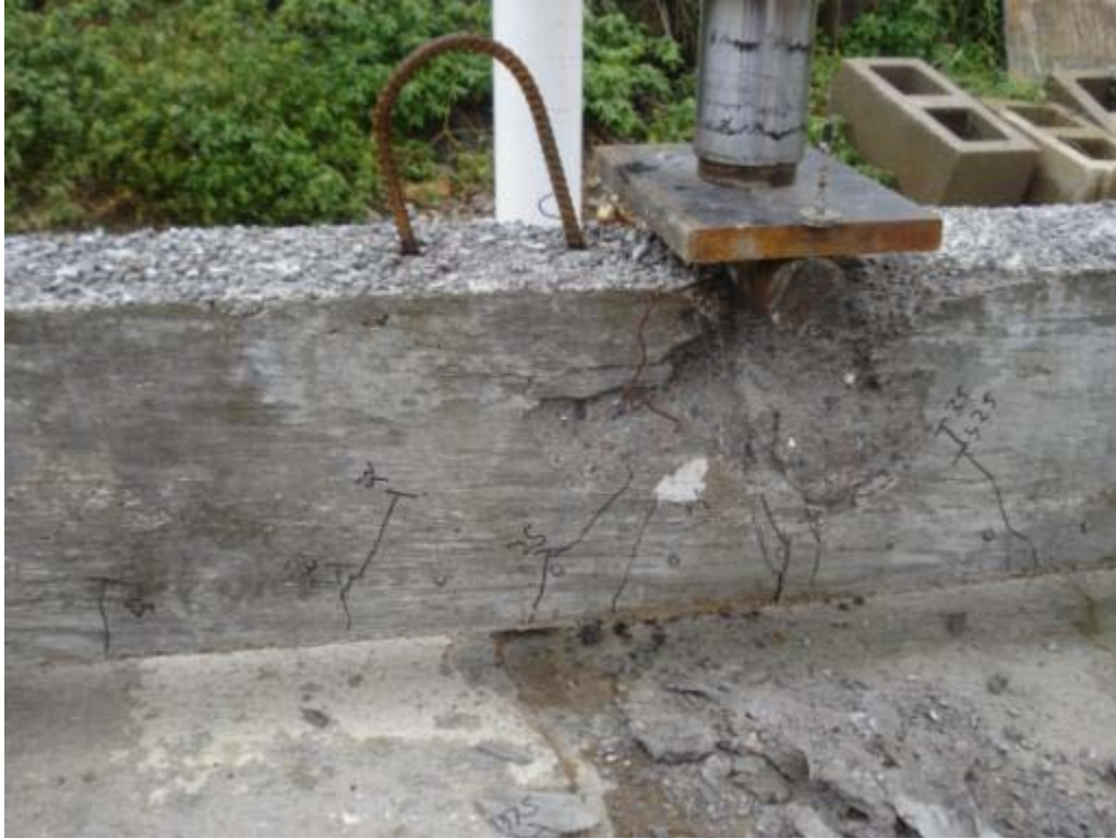
Figure 6.20: Cracking behavior and failure of specimen NSS-1L
