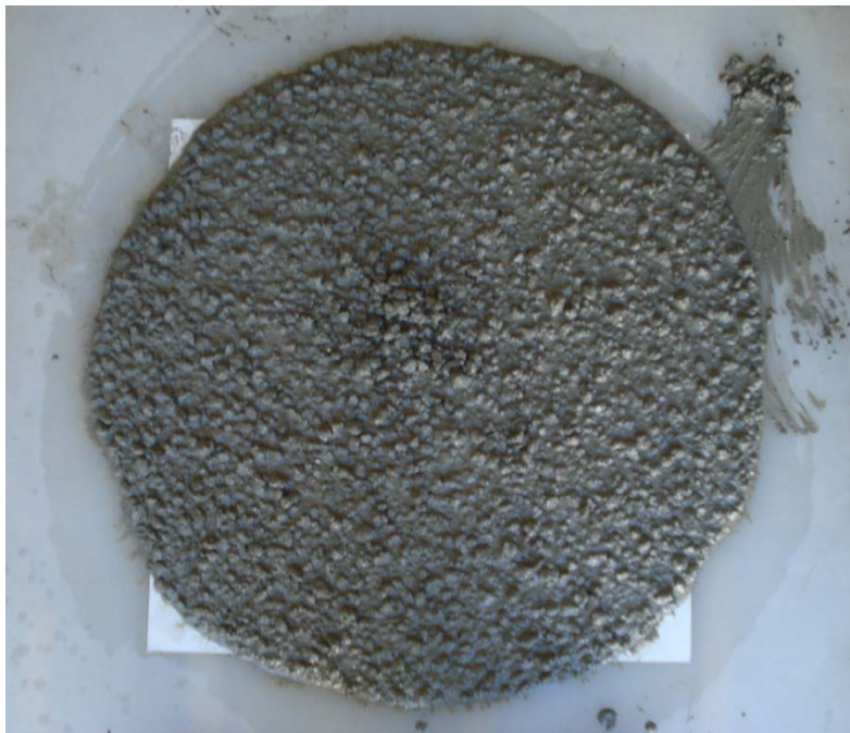
Figure 4.10: Slump flow of final HSC mixture
