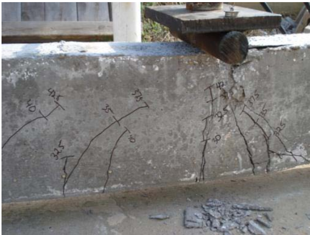
Figure 6.39: Cracking of specimen NSL-1L
