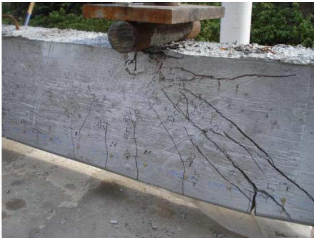
Figure 6.83: Cracking and failure of specimen HSS-4L
