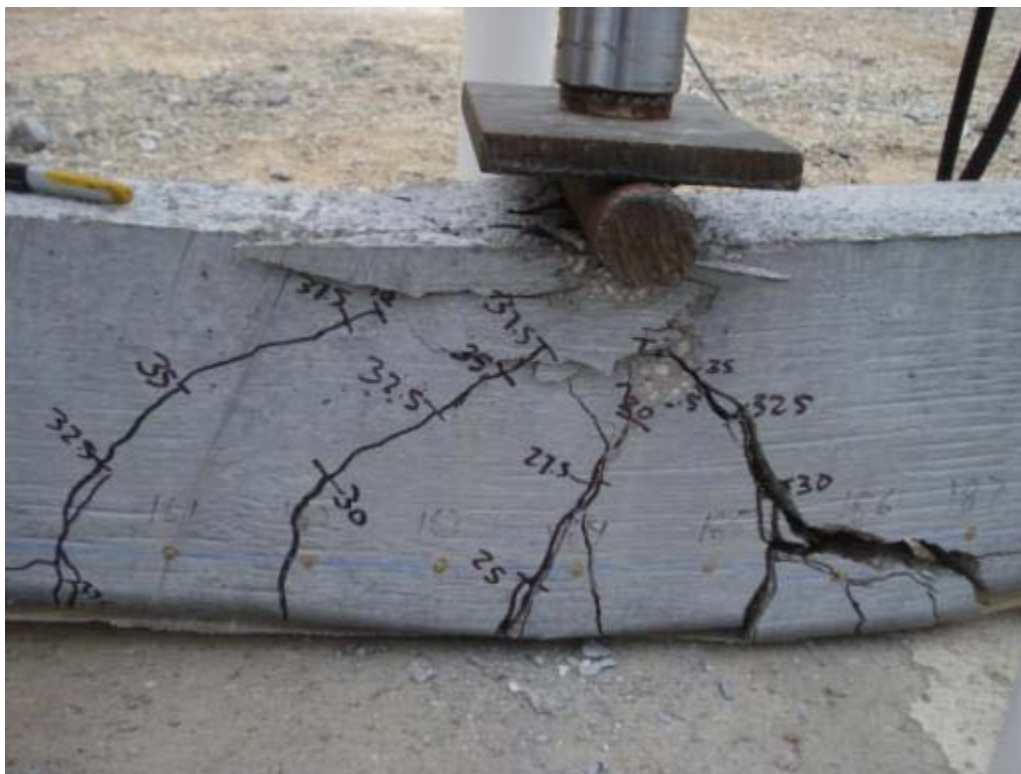
Figure 6.90: Cracking and failure of specimen HSL-2D
