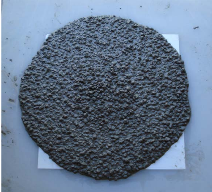
Figure 4.1: Slump flow of NSC mixture used to cast beams
