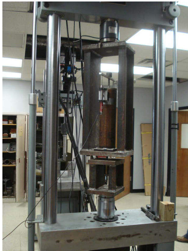
Figure 3.12: Setup for Standard Test for Strand Bond
