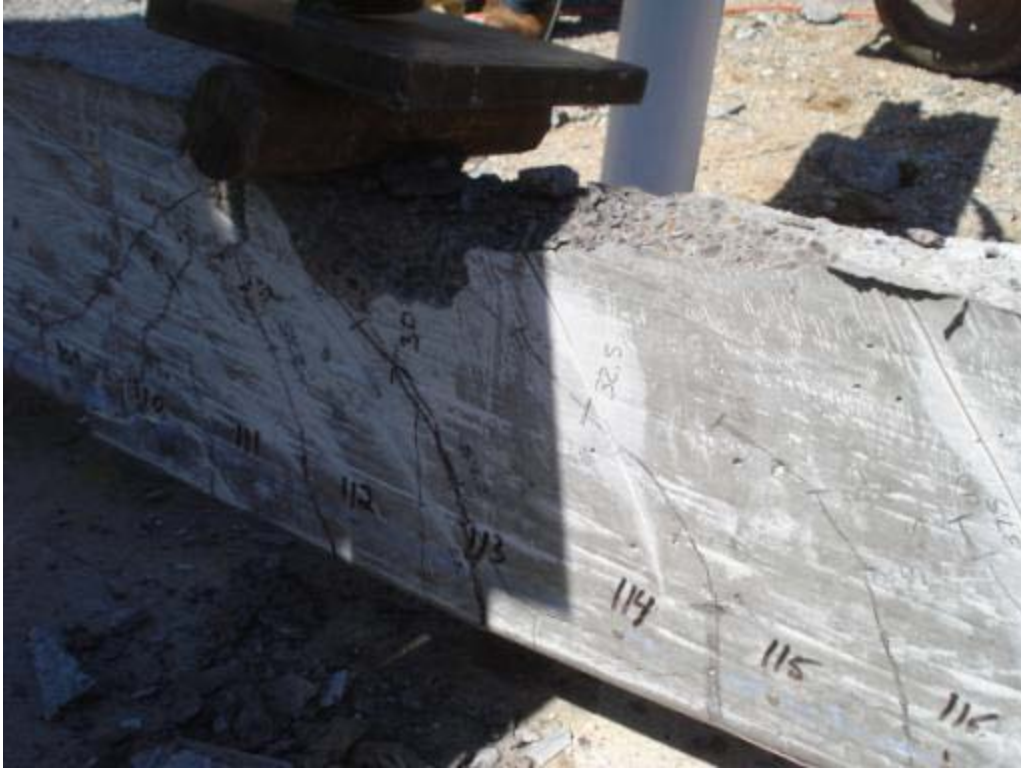
Figure 6.79: Cracking and failure of specimen HSS-3L
