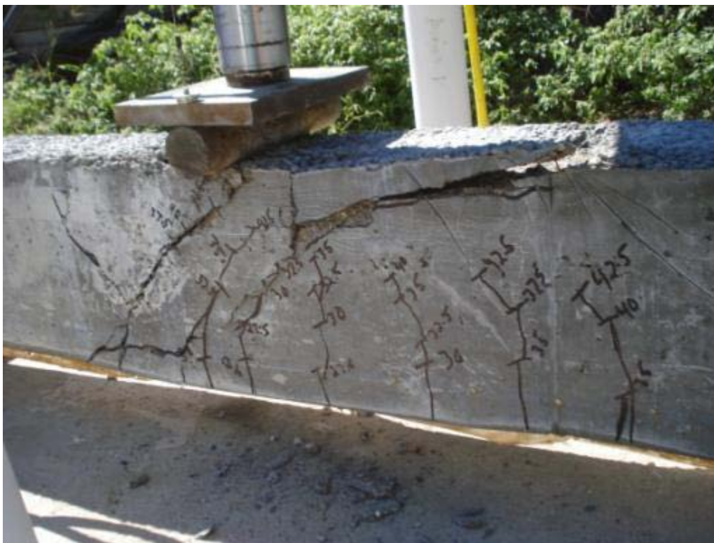
Figure 6.53: Cracking and failure of specimen HSC-1D
