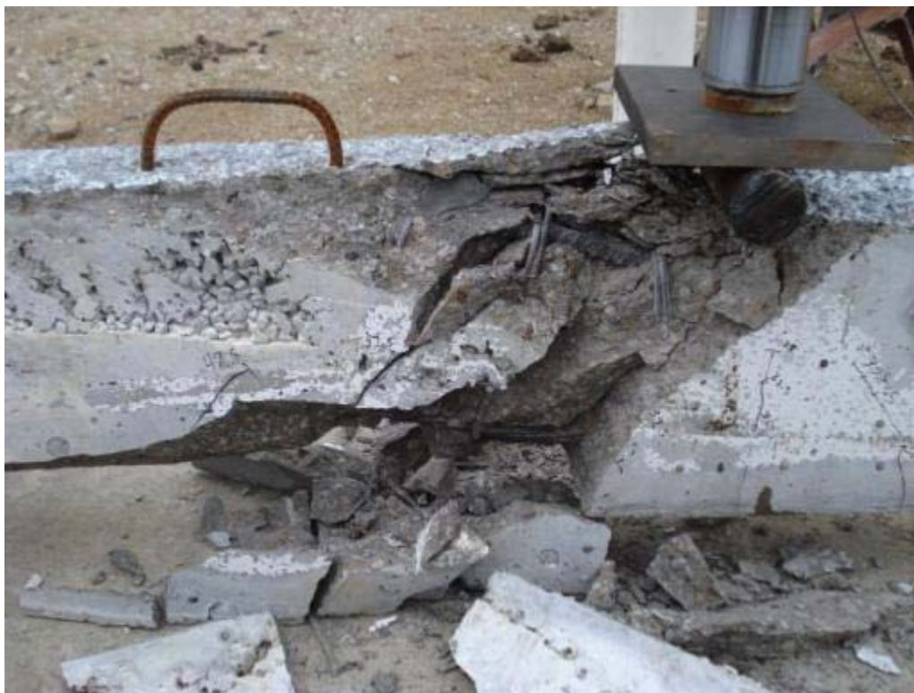
Figure 6.6: Failure of specimen NSC-2D
